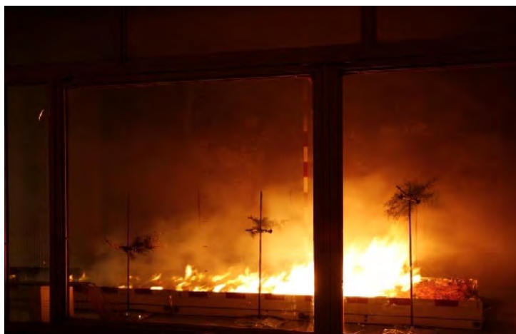
Fig. 8. An experimental fire in pine needles spreading below branches of Pinus halepensis and Cupressus sempervirens in the wind tunnel of the Mediterranean Agronomic Institute of Chania.
