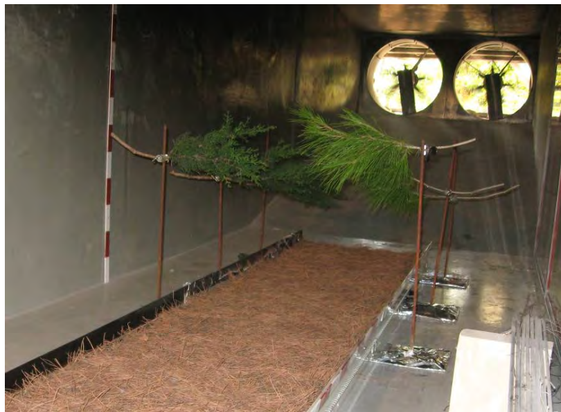
Fig. 7. An experimental setup in the wind tunnel of the Mediterranean Agronomic Institute of Chania to compare the ease of ignition of branches of Pinus halepensis and Cupressus sempervirens positioned above a flame front spreading in pine needles.
